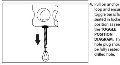
seated in locked position as seen in the **TOGGLE POSITION DIAGRAM.** The hole plug should be fully seated in drilled hole.
