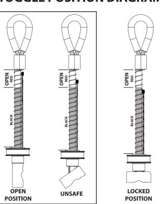
The indicator may be used as a means of determining toggle position when view of toggle bar is obstructed by the anchorage. If indicator is aligned with the red zone, toggle bar is in open or unsafe position. If top of indicator is below the red zone, toggle bar is in locked position.
