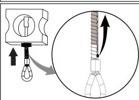
3. Push anchorage connector into drilled hole and engage toggle bar by pushing activator wire towards hole plug.
