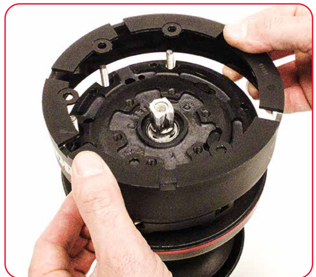
3. Replace the skirt on the base, pushing it into the correct position.
