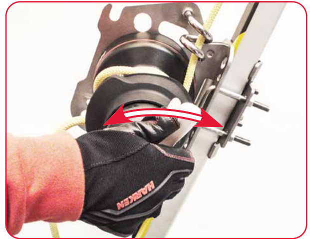
Check the correct operation of the semi-pulley control lever by turning and releasing it.
