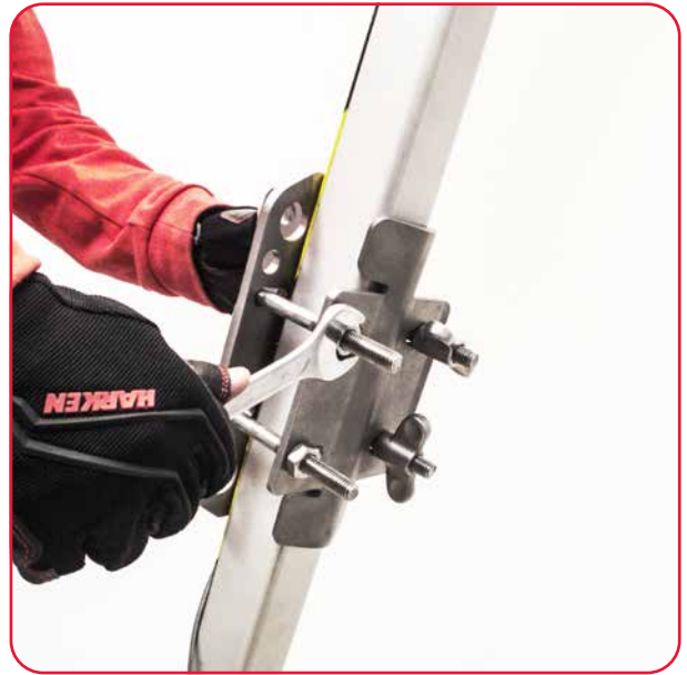
2. Tighten the two nuts with a wrench (30 Nm)
